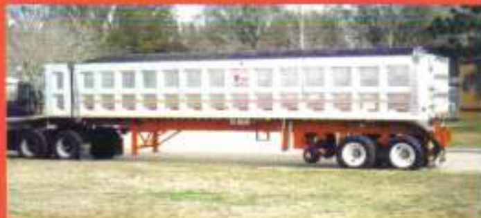
40' tri-axle frame-type, 35' dump body, 5' separate stationary blood tank, center gate, horizontal brace.
