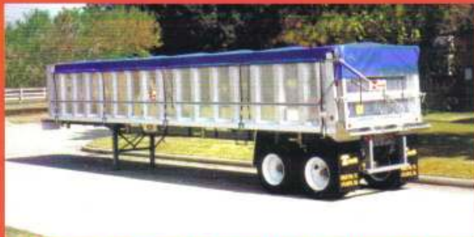
40' Frame-type tipper, no hoist, 850 gallon, internal blood tank, center gate, 8 floor drains, tarp, etc.
