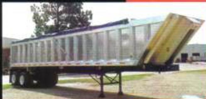
40' Frame-type with sloped nose and external hoist. Also, an 850 gal. internal blood tank, a manual center gate, floor clean outs and more.
