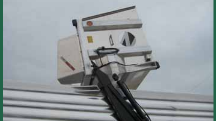
ALL-ALUMINUM BUCKET, WITH 4000 LB. LIFTING CAPACITY, DUMPS 18' INTO TRAILER
