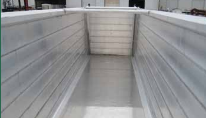
SMOOTH-SIDE, DUAL-WALL, ALL-ALUMINUM BODY AND FULL ALUMINUM FRAME
