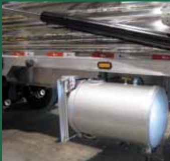
LARGE CAPACITY, PRESSURIZED WATER TANK AND HOSE
