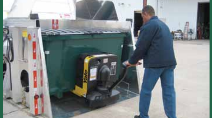
THE BUCKET ACCEPTS AN INDUSTRY STANDARD WASTE CONTAINER
